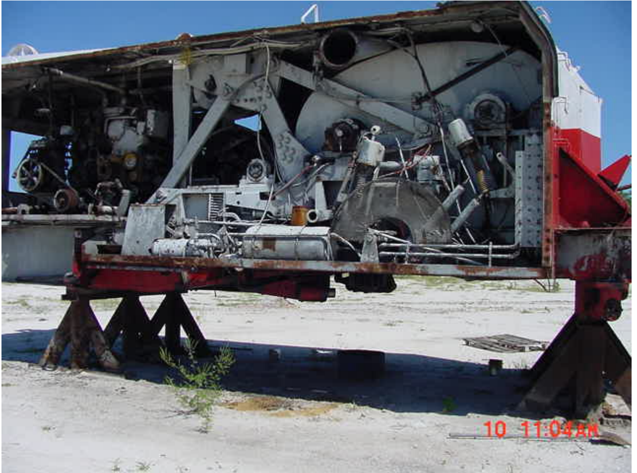
A dragline in pieces with stained soils and a container of petroleum underneath the engine compartment.
